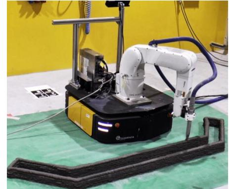
Figure 4 : The printing-while-moving robot
