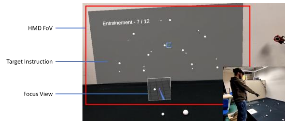
Fig. 4. View (HoloLens 2 and external) of a user pointing at a target on the horizontal surface: the red rectangle depicts the HMD FoV but is not visible by the user
