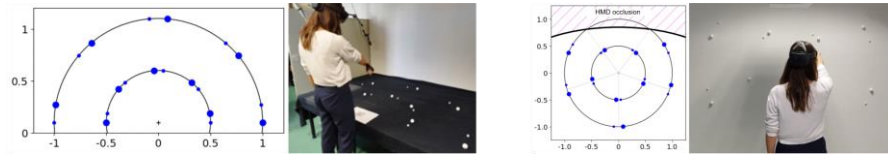
Fig. 3. Targets distribution on the horizontal (left) and vertical (right) surfaces (schematic and real).
